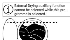
In the 6 kg Washing and 6 kg Drying programme, it is recommended to fill the machine to the level shown in the figure above for ideal drying conditions (you can see the level arrow when you open the loading door).
