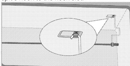
As shown in the figure, attach the rotisserie and skewer support wire into its place.
