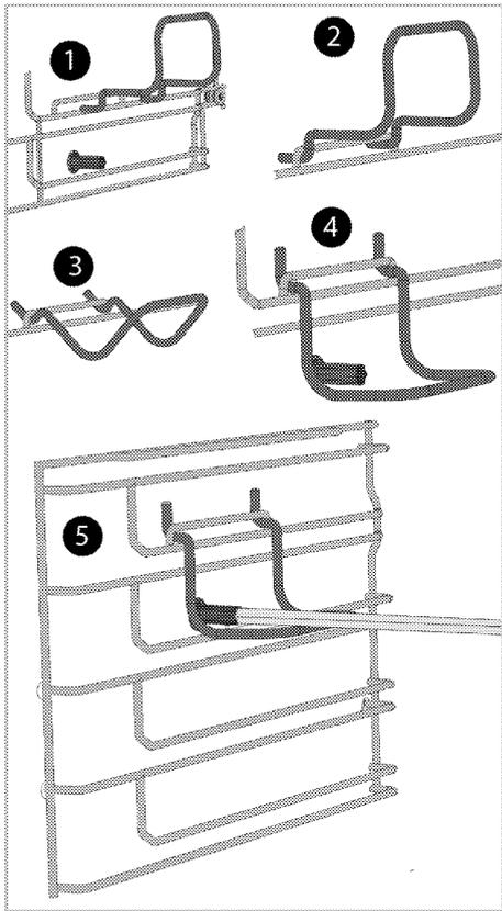
4. Place the pointed edge of the spit into the rotating slot on the left side inside the oven.
