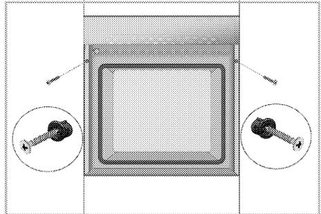
3. Make sure that the screws are tightened as required and that the oven does not move. There is a risk of tipping over during operation if the installation of the oven is not performed as per the instructions and the screws are not tightened as required.
