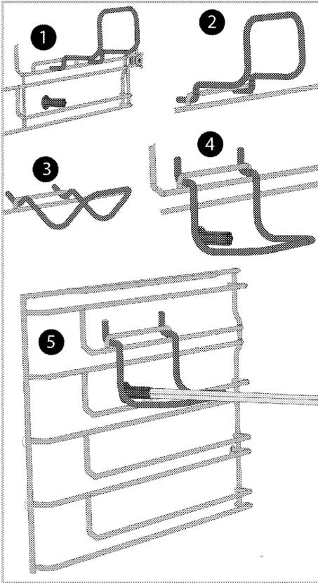
Place the pointed edge of the spit into the rotating slot on the left side inside the oven. If your spit has a plastic handle, remove it. As shown in the figure, hang the other edge of the spit onto the hook. Make sure the spit is secured with the hook, as in the figure.
