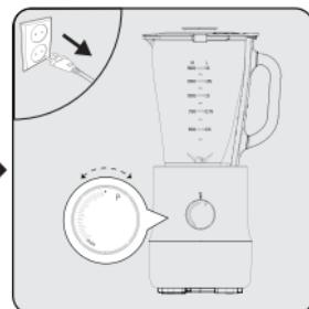
When mixing is complete, turn the speed adjustment knob (7) to the "0" position and remove the plug from the socket.
