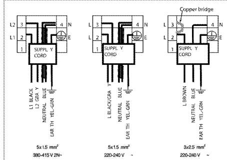
2. For single-phase connection, connect the wires as identified below:
