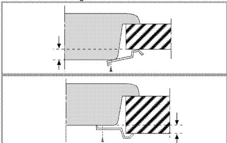
**i** When installing the hob onto a cabinet, a shelf must be installed in order to separate the cabinet from the hob as illustrated in the above figure. This is not required when installing onto a built-under oven.
