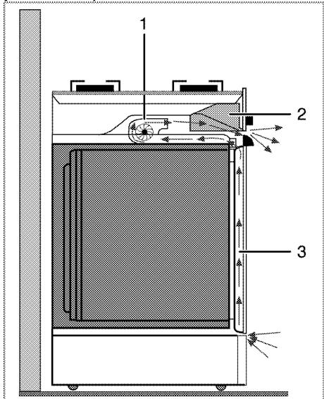
1 Cooling fan (Rashladni ventilator)
