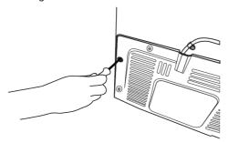
Attach 2 plastic wedges on the ventilation cover as shown in the figure.
