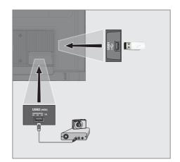
Connect the USB2 (HDD) interface of the television and the corresponding socket on the data device (external hard drive, digital camera, card reader or MP3 player) using a USB cable;
