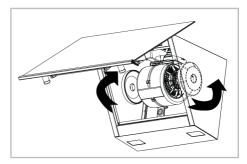
Place the lug slots of your new carbon filters into the lugs on the motor holder and turn them clockwise to snap them into place.
