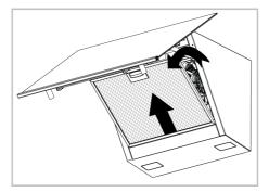
Reinstall the aluminium filter in its slot after flushing by following the above steps in reverse.
