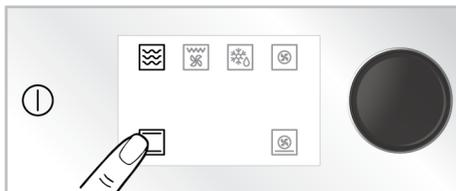
4. The pre-set temperature for the operating function you selected appears on the display. Turn the oven control knob to the right/left to change this temperature.
