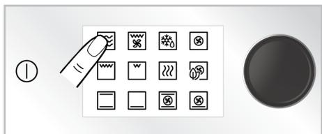
3. Touch the %W key to change the microwave power level. Adjust the desired microwave power by turning the oven control knob to the right/left.
