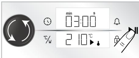
⇒ Your oven will start operating immediately at the selected combi function, temperature and microwave power. The adjusted baking time starts to count down. On the display, the  $\text{▶}$  and  $\text{↓}$  symbols are shown. When the baking time is completed, "End" text appears on the display, audible warning is given and baking stops.
