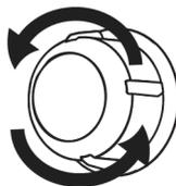
3. If your oven lamp is type (A) shown in the figure below, rotate the oven lamp as shown in the figure and replace it with a new one. If it is type (B) model, pull it out as shown in the figure and replace it with a new one.
