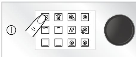
3. Touch on the combi function you want to cook with the microwave function. Both will activate. (e.g. Microwave + Top and bottom heating)
