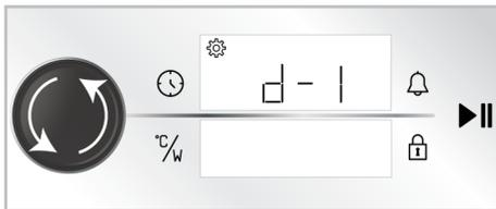
3. Activate the brightness setting by touching the ⌚ key again or pushing the oven control knob once.
