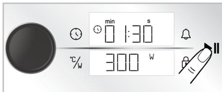
⇒ Your oven will start operating immediately in microwave function and power. The adjusted baking time starts to count down. On the display, the ► and W symbols are shown. When the baking time is completed, "End" text appears on the display, audible warning is given and baking stops.
