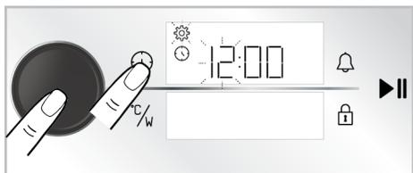
3. Set the time of day by turning the oven control knob to right/left and activate the minute field by pushing the oven control knob once or touching the
