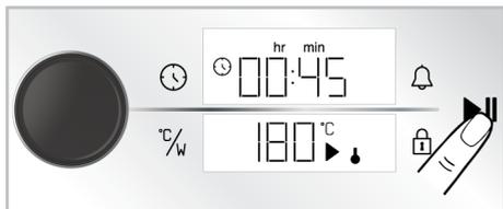
⇒ Your oven starts operating immediately at the selected operating function and temperature and the baking time countdown appears on the display. On the temperature display, the ↓ and ► symbols are shown. As the oven inner temperature reaches the set temperature, each stage of the ↓ symbol will light up. When the adjusted baking time is completed, “End” text appears on the temperature display, the timer gives an audible warning and baking stops.
