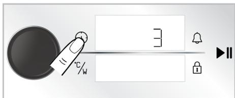
2. Activate the timer field by pushing the oven control knob once or touching the
