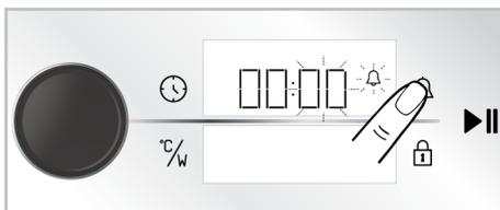
2. First set the minutes by turning the oven control knob to the right/left and activate the timer field by touching the
