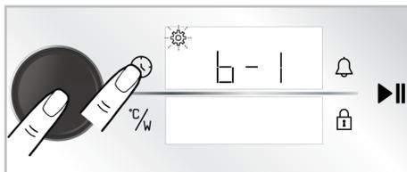
4. Adjust the desired tone by turning the oven control knob to the right/left.
