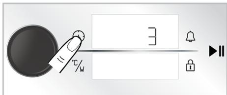
2. Activate the timer field by pushing the oven control knob once or touching the ⌚ key once.
