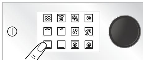
3. The pre-set temperature for the operating function you selected appears on the display. To change this temperature, push the oven control knob once or touch the °C key and turn the oven control knob to the right/left.
