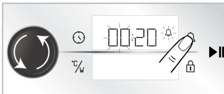
⇒ On the timer/duration display, the
