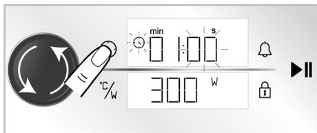
8. Adjust the baking time in seconds by turning the oven control knob to the right/left.
