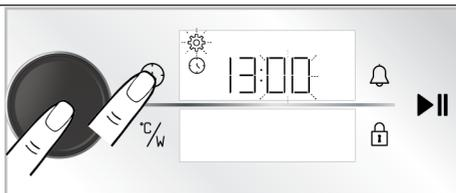
4. Set the minute by turning the oven control knob to right/left. Approve the setting by pushing the oven control knob once or touching the
