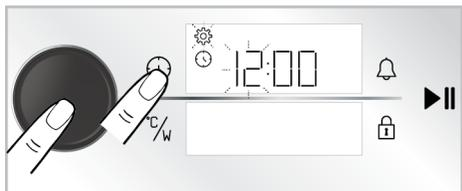
3. Set the time of day by turning the oven control knob to right/left and activate the minute field by pushing the oven control knob once or touching the ⌚ key once.
