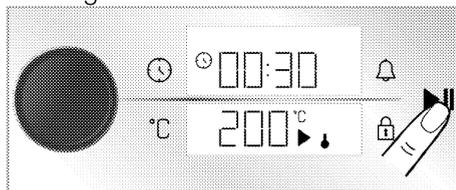
13. At the end of the cooking time, the audible warning sounds for one minute. If the ① key is touched, the oven turns off. If any key other than these keys is touched, the audible warning will stop.
