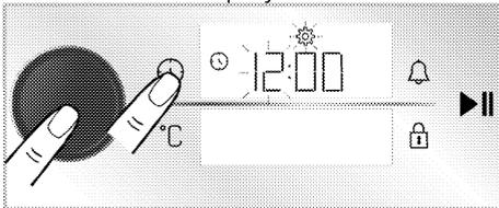
3. Set the hour by rotating the oven control knob to right/left and press the control knob to right/left and press the
