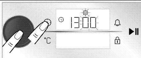
4. Set the minute by rotating the oven control knob to right/left. Confirm the time setting by pressing on the oven control knob or touching
