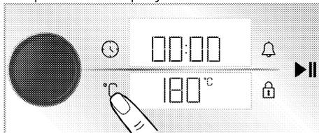
6. Press oven control knob or touch the ⌚ key once for setting the cooking time.
