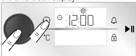
3. Set the hour by rotating the oven control knob to right/left and press the oven control knob or touch
