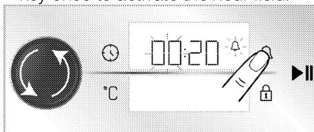
3. Set the hour by rotating the oven control knob to right/left. Confirm the time setting by pressing on the oven control knob or touching
