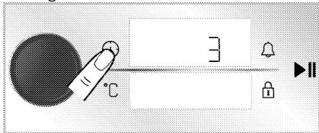
2. Rotate the oven control knob to right/left until the
