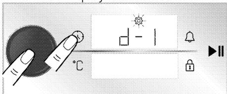
4. Set the desired brightness level by rotating oven control knob to right/left.
