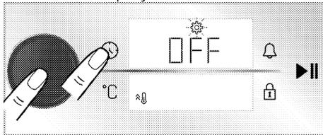
4. Rotate the oven control knob to right/left to change the "OFF" setting displayed on the time/clock display to the "ON" setting.
