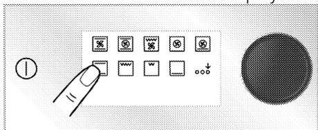
3. Touch on the operating function you want to cook on function display. If the function you want to select is not among the first operating functions that appear on the function display, you can activate the lower row of operating functions by touching on "Extra function activation".
