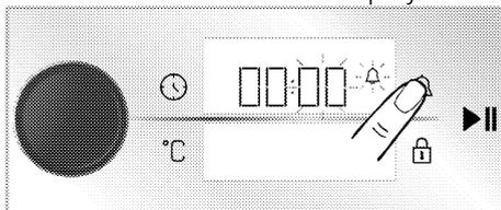
2. Set the minute by rotating the oven control knob to right/left and touch
