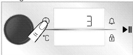
2. Press the oven control knob or touch
