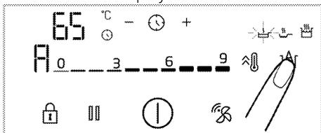
2. On the timer display, "65" is displayed as the lowest temperature setting for the setting of low temperature. By touching the
