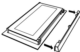
3. As shown in the figure, gently lift the innermost glass (1) towards "A" and then, remove it by pulling towards "B".
