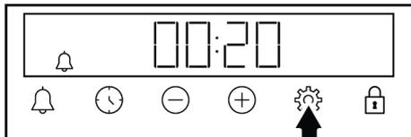
⇒ After setting the alarm time, the
