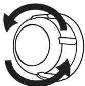
3. If your oven lamp is type (A) shown in the figure below, rotate the oven lamp as shown in the figure and replace it
