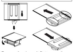
To group the wine rack, first remove the glass shelf from the refrigerator. Place it on the glass shelf by pushing the plastic part through the front and back grooves as shown in the picture. The product will be ready to use with the foldable wine rack.
