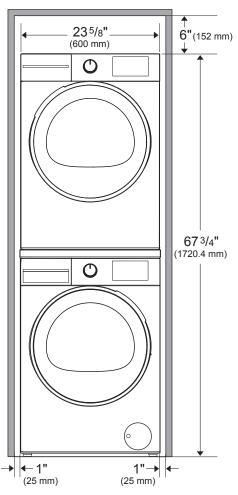
NOTE: Only one electrical outlet is needed since the washer can plug into the dryer. The use of two electrical outlets may be used as an alternative.
