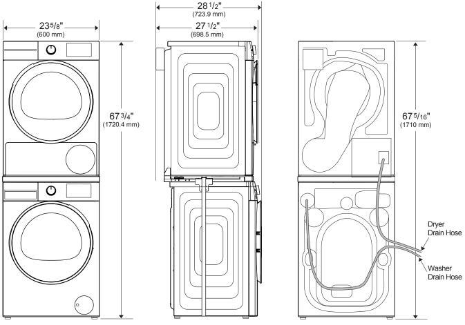
NOTE: Only one electrical outlet is needed since the washer can plug into the dryer. The use of two electrical outlets may be used as an alternative.
