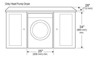
Required Minimum Clearances: (Stand Alone, Side by Side, or Stacked)
