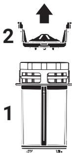
4. Clean all three filters under tap water by means of a brush.
